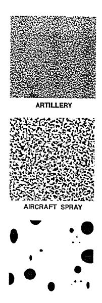
MISSILE Figure 1-3. Heavy liquid contamination on M9 paper (10 grams/square meter).
